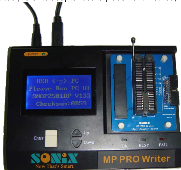
Figure 2-1 MP PRO Writer hardware connection
