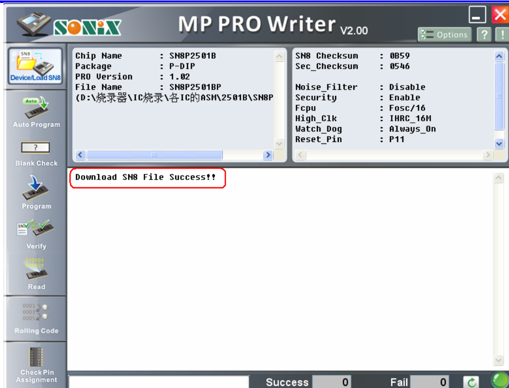
Figure 3-6 firmware update completed, SN8 download successfully
