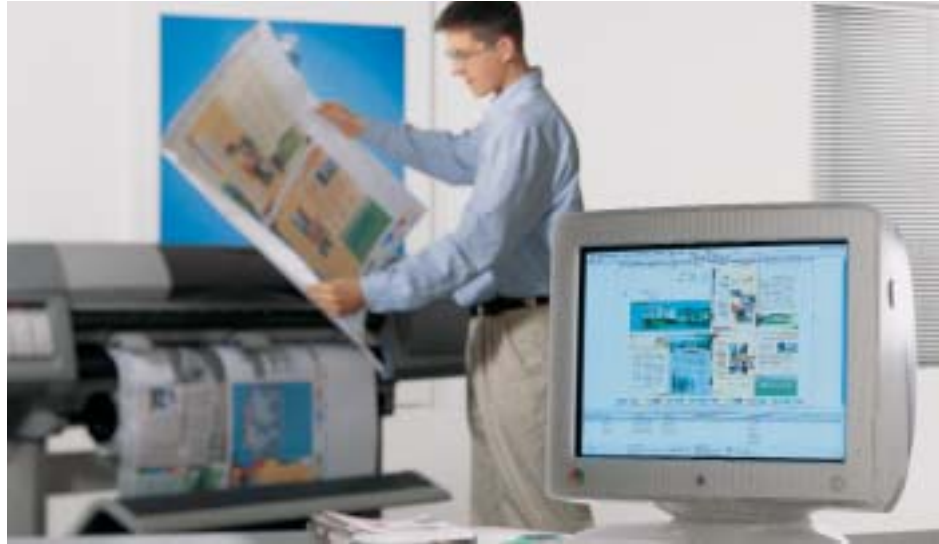
There is a long way to go to the final print product. The process involves many intermediate steps such as the proof shown here. Throughout all the steps leading from one color space to the next, professional color management ensures optimum color reproduction on the respective output devices.
