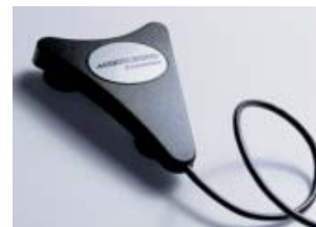
The colorimeter for monitor calibration is able to operate without its own light source and is therefore significantly smaller than a spectrophotometer.
