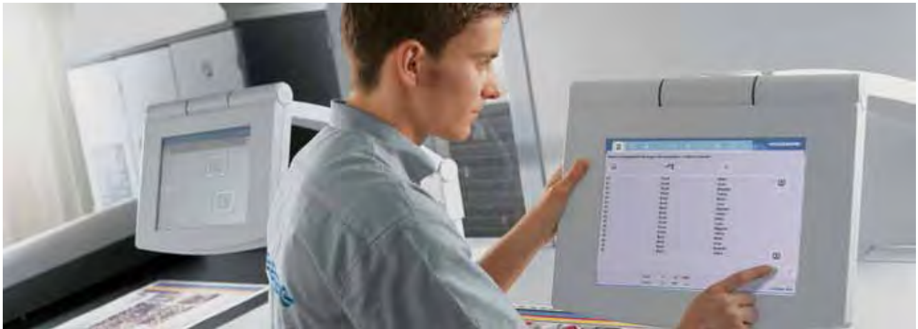
Plate production can be controlled from the prepress stage as well as from the Prinect CP2000 Center. Starting with version 41, individual plate outputs can be repeated from the Center.
